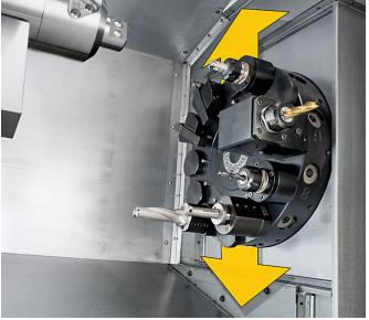
The 'Y' axis of the XYZ CT 65 LTY can travel 35mm above and below centreline (70mm total travel), making easy work of most components that would normally require milling and turning operations.
